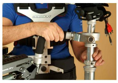
gimbal. All five fingers should be LIGHTLY in contact with the post. This hand will point the camcorder and do pans and tilts.
